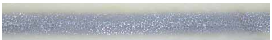
Open-pore Lauramid Hybrid®: Lauramid® penetrates completely into the aluminium foam
