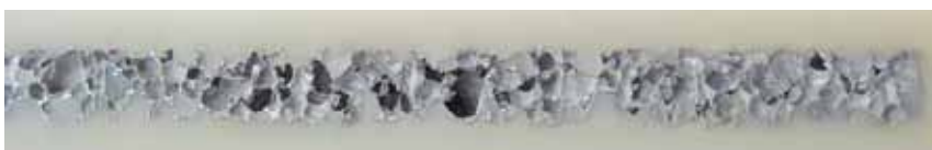
Closed-pore Lauramid Hybrid®: Lauramid® penetrates into the outer pores of the aluminium foam
