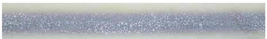
Closed-pore Lauramid Hybrid®: Lauramid® penetrates into the outer pores of the aluminium foam
