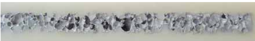
Closed-pore Lauramid Hybrid®: Lauramid® penetrates into the outer pores of the aluminium foam
