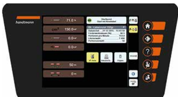
↑ Setting parameters at vacuum filler deactivated, operation at clipper
