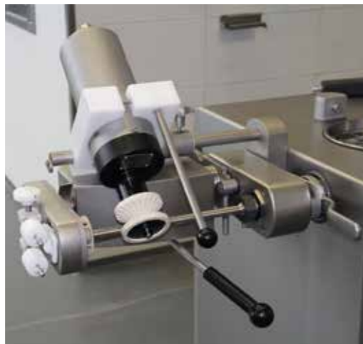
↑ 78-6 casing spooling device
