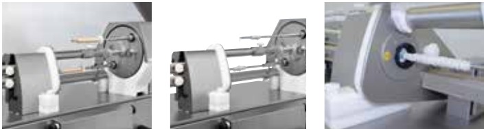
↑ Casing spooling with semi-automatic casing change function
