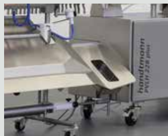
↑ Collection tray in cleaning position
