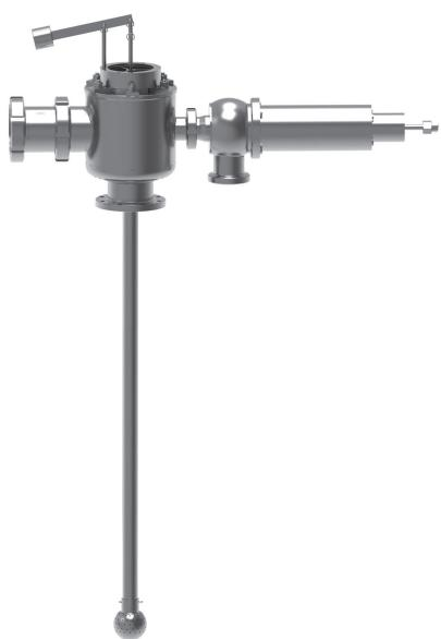
Tanks or containers are often equipped with a combined CIP/gas tank line. This ends at the tank in a cleaning air/value combination (RLV combination) equipped with a tank connection. This compact multifunctional unit controls the supply of CIP fluids or the supply and removal of the gas flows / CO<sub>2</sub> via an integrated switching valve. This guarantees safe media management.
