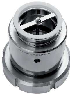
These valve types are designed for underpressure protection of smaller and medium-sized containers. They can be installed as a single valve or in combination with a cleaning unit (RLV). These vacuum valves can be installed in the upright (vertical) position and the spring-loaded version can also be installed in the horizontal position.
