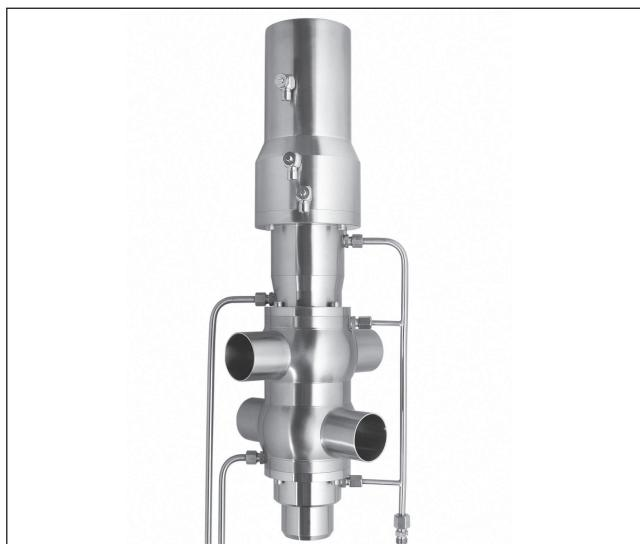
Double-seat valves can be installed as single valves or in a valve group (valve block) and form the interface between separate pipe systems.
