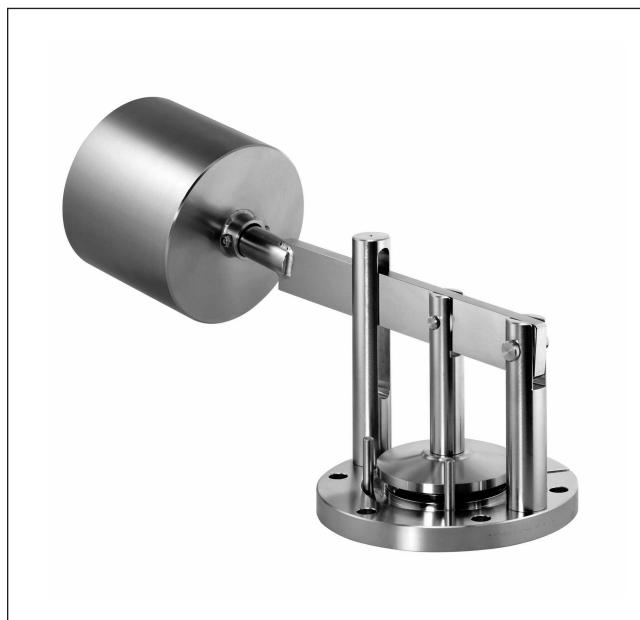
This valve type is specially designed for overfill protection of large containers and can be installed as a single valve or in combination with a tank dome cap. These safety valves can only be used in the upright (vertical) position. The sophisticated construction allows safe, hygienic operation.
