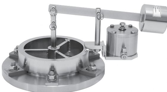
This valve type is specially designed for underpressure protection of large containers and can be installed as a single valve or in combination with a tank dome cap. These vacuum valves can only be used in the upright (vertical) position. The sophisticated construction allows safe, hygienic operation.
