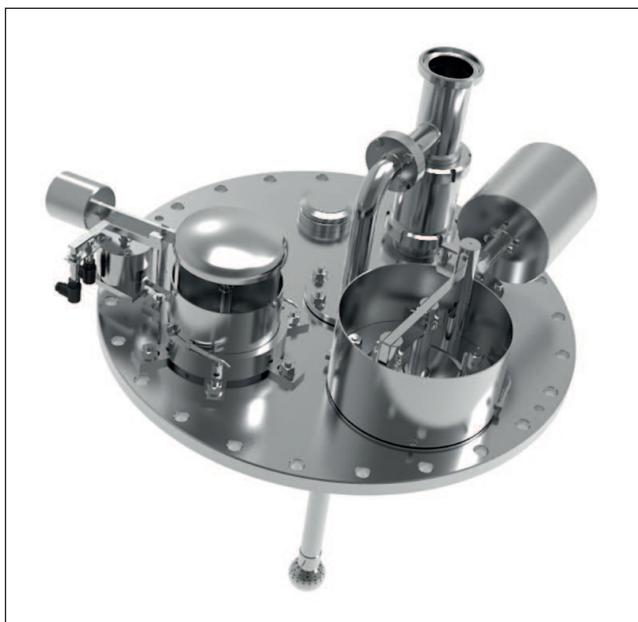
Dome caps are modularly constructed functional units born from many years of experience in armature and plant construction. They are equipped with high-quality armatures and measurement equipment for pressure protection, supply and removal of CO<sub>2</sub>, CIP cleaning and process monitoring. Dome caps are predominantly used with large cylindroconical tanks (ZKT).
