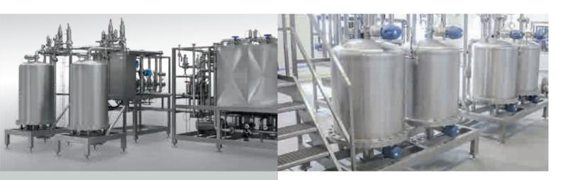
The CSS consists of one or several modules which are completely filled with the adsorbent. The adsorbent is permanently retained between an inlet and an outlet screen, making the dosing of precoat and feed suspension prior to each stabilization unnecessary.
