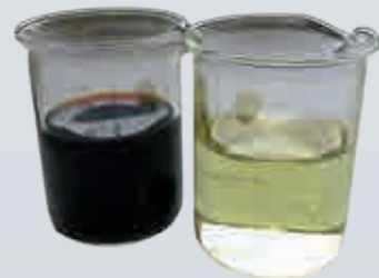
↑ Colour removal from caustic from regeneration processes
