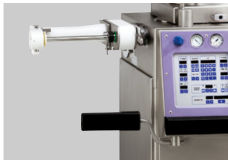
Holding device 60-8 One special feature is gentle linking of natural casing. This unit proves particularly useful for frequent product changes.
