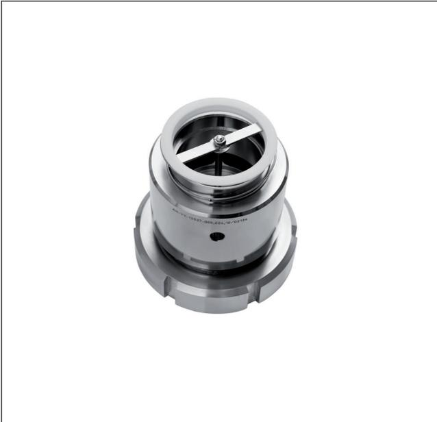
These valve types are designed for underpressure protection of smaller and medium-sized containers. They can be installed as a single valve or in combination with a cleaning unit (RLV). These vacuum valves can be installed in the upright (vertical) position and the spring-loaded version can also be installed in the horizontal position.
