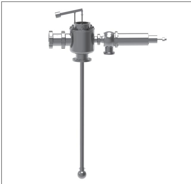
Tanks or containers are often equipped with a combined CIP/gas tank line. This ends at the tank in a cleaning air/valve combination (RLV combination) equipped with a tank connection. This compact multifunctional unit controls the supply of CIP fluids or the supply and removal of the gas flows / CO<sub>2</sub> via an integrated switching valve. This guarantees safe media management.
