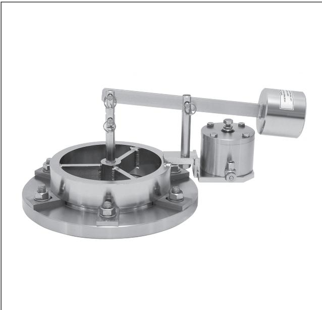
This valve type is specially designed for underpressure protection of large containers and can be installed as a single valve or in combination with a tank dome cap. These vacuum valves can only be used in the upright (vertical) position. The sophisticated construction allows safe, hygienic operation.
