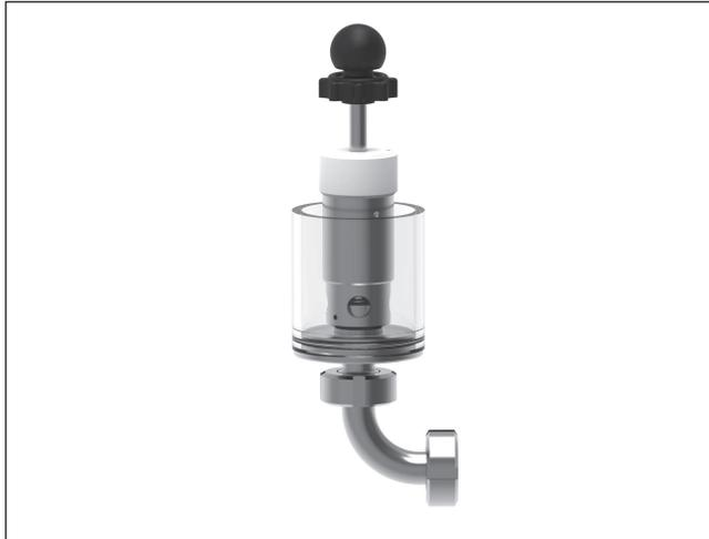
CO<sub>2</sub> gas develops constantly during fermentation. The regulated drainage was traditionally effected via bunging devices. This makes it possible to maintain the necessary pressure inside the tank for the fermentation process constant.
